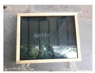
Fig.1 Flat plate collector used in the experiment
