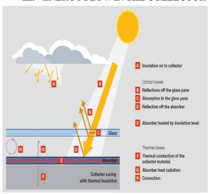
Fig.8 Energy flow in the collector
