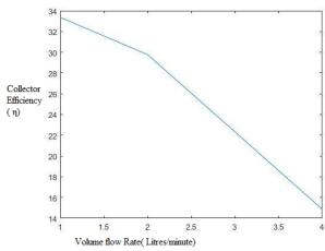
Fig.9 Variation of Collector efficiency with volume flow rate
